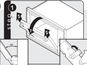
Open door approximately 20°, then slowly pull upward until the door stop pops out of door socket.
